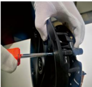
2. Rotate the mounting bracket to the left.
